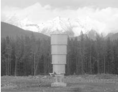
The Canadian Rockies loom over a gas flare burner at an exploratory CBM well in the upper Elk Valley.
